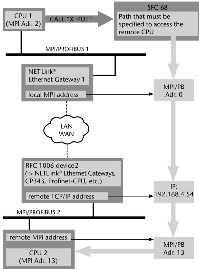
If the intention is to expand an already configured X\_PUT/X\_GET process via TCP/IP, it is only necessary to include an additional X\_PUT (with the parameters for the remote station -> see illustration) in the program execution to open the communication channel via the NETLink®.
