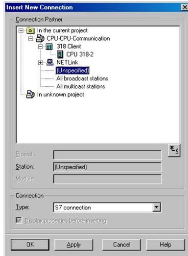
When configuring the S7 connection, make sure that the right IP address is being assigned. Enter the NETLink® adapter's IP address as the "Partner's" IP address.
