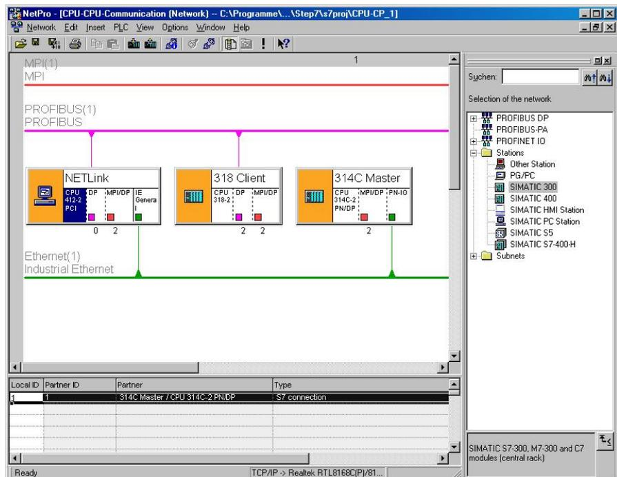
8. Communications in the PG/PC interface must be managed by the local network adapter.
