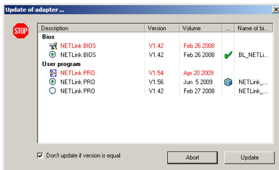
To perform an update from a firmware version lower than V1.42 to a version higher than V1.42, it is first necessary to update to version 1.42 as an intermediate step.
