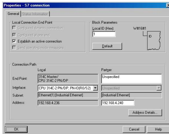
In addition, make sure the correct “Rack / Slot” and “Connection Resource” is assigned.
