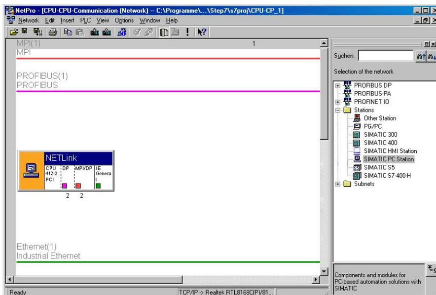
You will now have to configure the settings for “NETLink.” A dialog box in which you will have to configure the “Industrial Ethernet” settings for the NETLink® unit will appear (IP address/subnet mask). In addition, you will have to configure the subnet (“Industrial Ethernet”) to which the NETLink® unit is also connected.
