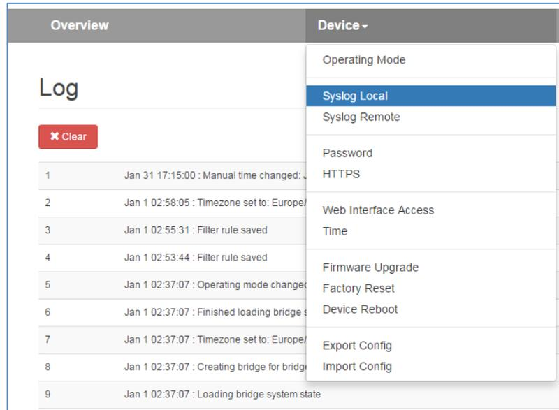
The screenshot shows the 'Log' configuration page. On the left, there is a 'Log' section with a 'Clear' button and a table of recorded events. On the right, there is a 'Device' menu with various options, including 'Syslog Local' which is currently selected.
