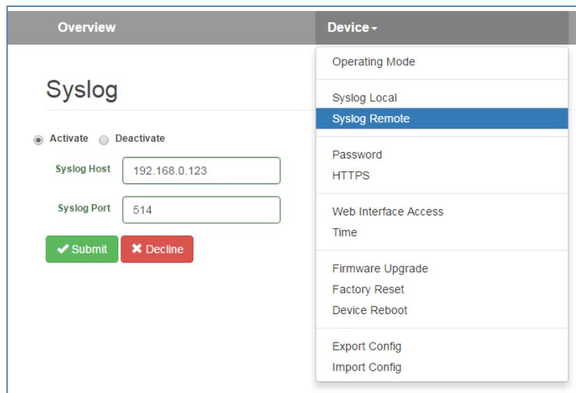
The screenshot shows the 'Syslog' configuration page. On the left, there is a 'Syslog' section with 'Activate' and 'Deactivate' radio buttons, and input fields for 'Syslog Host' (192.168.0.123) and 'Syslog Port' (514). There are 'Submit' and 'Decline' buttons. On the right, there is a 'Device' menu with various options, including 'Syslog Remote' which is currently selected.
