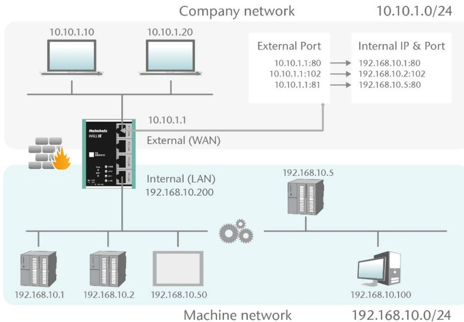
In the following example, the website (Port 80) of the CPU with the IP 192.168.10.5 via WAN can be reached through access to the WALL IE-own IP address 10.10.1.1 with Port 81.
