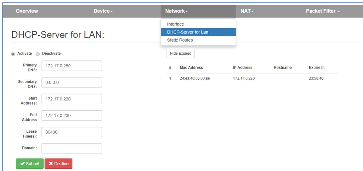
**Primary/Secondary DNS:** Specifies the IP address of a DNS server that is available to a DHCP client.
