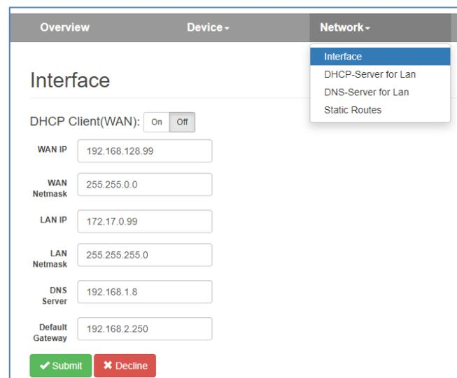
It is necessary to indicate a DNS server for the SNTP service (see ch. 11.8).
