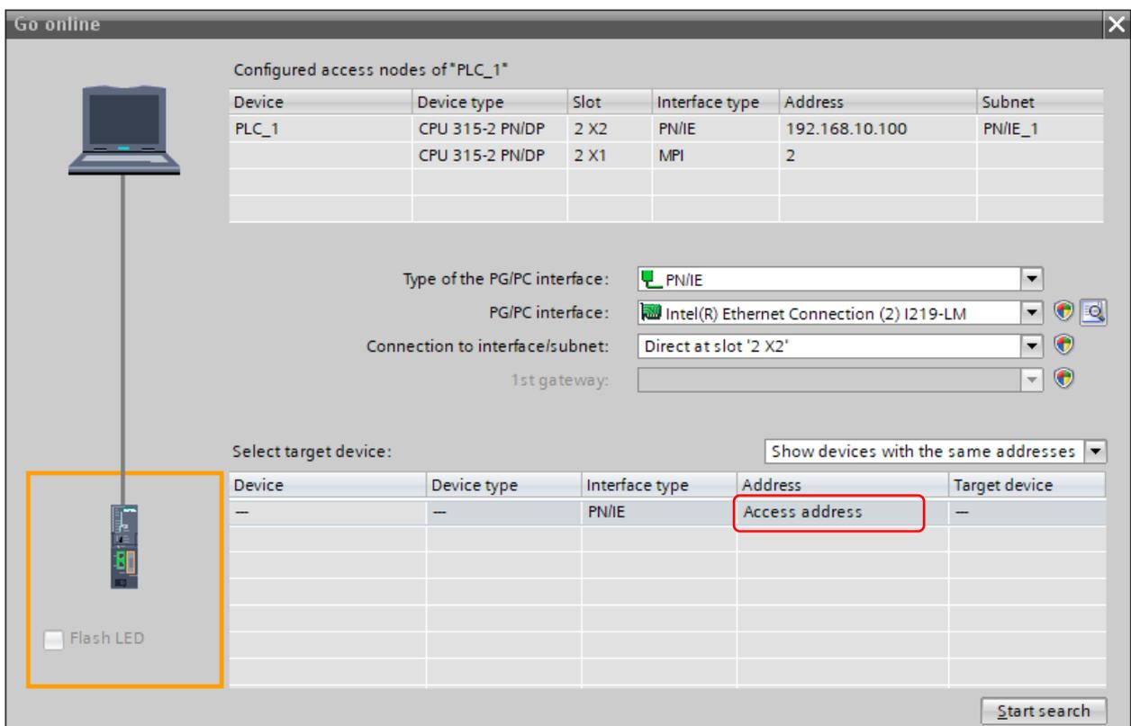
Click on "Access Address" and enter the WAN IP address specified for the device (CPU) in the WALL IE in Basic NAT. Confirm the entry by clicking on the window. An attempt is now made to establish a connection using the entered IP address.
