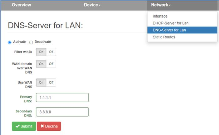
The screenshot shows the 'DNS-Server for LAN' configuration page. At the top, there are tabs for 'Overview', 'Device', and 'Network'. The 'Network' tab is active, and a dropdown menu is open, showing options: 'Interface', 'DHCP-Server for Lan', 'DNS-Server for Lan' (which is highlighted), and 'Static Routes'. The main content area is titled 'DNS-Server for LAN:' and contains the following settings:
