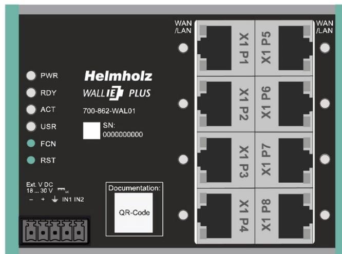
A reset to factory settings can be initiated with the function button (FCN) (see ch. 12). The reset button (RST) initiates a restart of the WALL IE PLUS.
