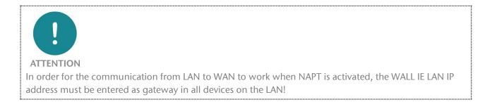
If the **NAPT** option is deactivated, the query packets from the LAN are forwarded from the LAN to the WAN with their original sender IP and sender port.
