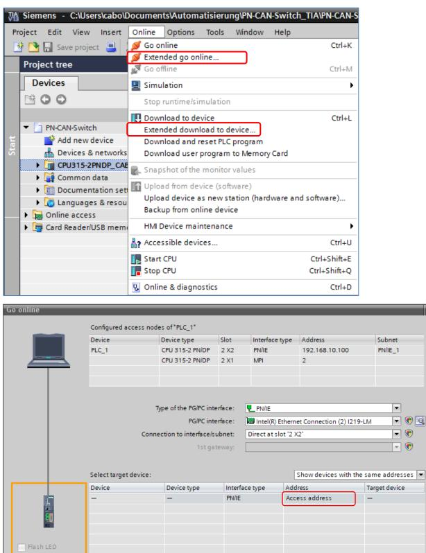
Click on "Access Address" and enter the WAN IP address specified for the device (CPU) in the WALL IE in Basic NAT. Confirm the entry by clicking on the window. An attempt is now made to establish a connection using the entered IP address.
