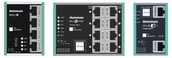
The **NAT operating mode** serves the forwarding of the data traffic between various IPv4 networks. It enables the address translation via NAT and uses packet filters for the limitation of access to the automation network located behind.
