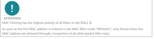
When MAC Filtering is used in the "Whitelist" mode, the MAC addresses of **all** allowed devices must be indicated.
