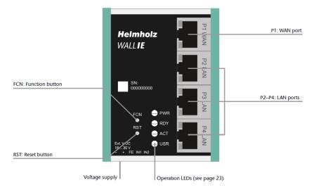
A reset to factory settings can be initiated with the function button (FCN) (see ch. 12). The reset button (RST) initiates a restart of the WALL IE.
