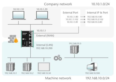
In the following example, the website (Port 80) of the CPU with the IP 192.168.10.1 via WAN can be reached through access to the WALL IE-own IP address 10.10.1.1 with Port 81.
