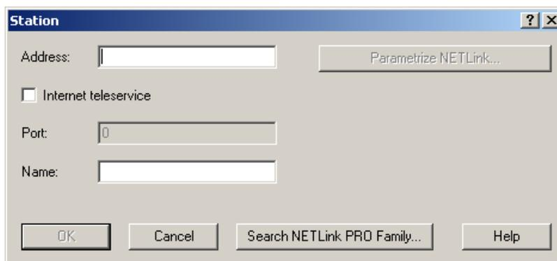
To be able to access a NETLink® with the NETLink-S7-NET driver, a station must be set up first. This station is virtual and is not stored in the NETLink® Gateway hardware – it permits easier differentiation if several NETLink® devices from the NETLink® family are used.
