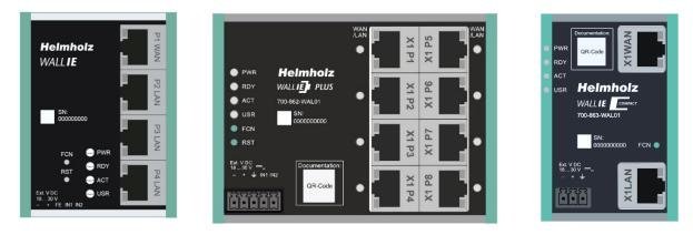
The **NAT operating mode** serves the forwarding of the data traffic between various IPv4 networks. It enables the address translation via NAT and uses packet filters for the limitation of access to the automation network located below.
