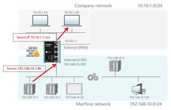
The option "**NAPT: Active**" thus enables communication of devices from the LAN with devices in the WAN. WALL IE thereby acts as a gateway to administer the implementation to the IP addresses of the WAN network and looks after the assignment of the response.
