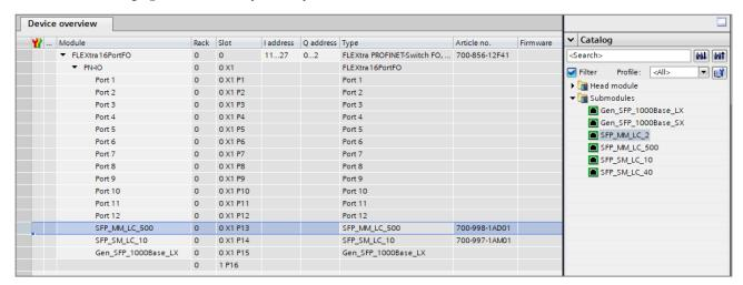
If the Helmholz SFP modules are configured, the FLEX tra PROFINET switch checks whether exactly the configured SFP module has been plugged into the specified port. If an SFP module is missing or an SFP module of a different type is plugged, a diagnosis is triggered. Thus a wrong configuration or a wrong cabling can be detected easily.
