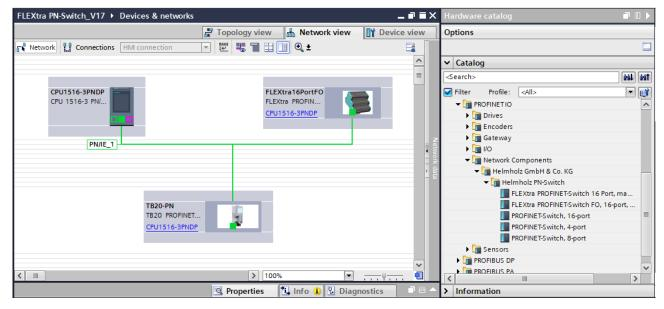
By calling up the object properties, you must give the FLEXtra PROFINET switch a unique PROFINET name in the project and check the IP address for plausibility.
