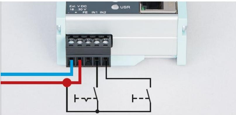
The inputs IN1 and IN2 have no function in the current firmware version yet and will be available for possible additional functions in a later firmware version.
