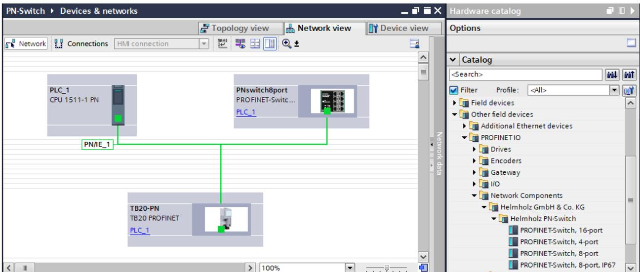
By calling up the object properties, you must assign the PROFINET switch a unique PROFINET name in the project and check the IP address for plausibility.
