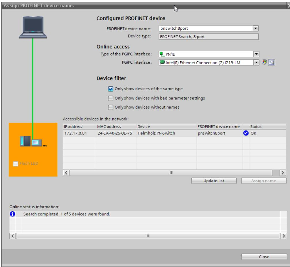
The clear identification of the PROFINET switch is ensured here by the MAC address of the device. The MAC address of the device can be found on the device front of the PROFINET switch.
