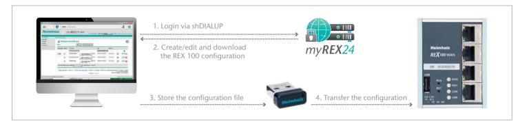
Use the USB-based parameter configuration method if the REX 100 router cannot be reached either through the local network (LAN) or through the Internet.
