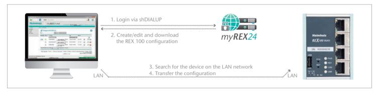
In order to be able to transfer the configuration through the LAN network, it must be possible to reach the REX 100 unit (the one being configured) in the same network in which the computer with the shDIALUP software is also found.
