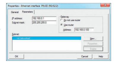
In order to be able to reach the PLC through the VPN tunnel, you will have to select the appropriate Open VPN adapter in the PG/PC interface. The virtual network connection responsible for this is the TAP Windows¹ Adapter V9.
