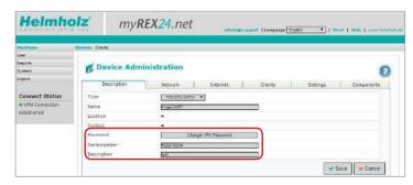
All REX 100 routers come with a LAN-side IP address of 192.168.0.100/24 as a default. Modify the IP address and the subnet mask in keeping with the specifications from the machinery network.
