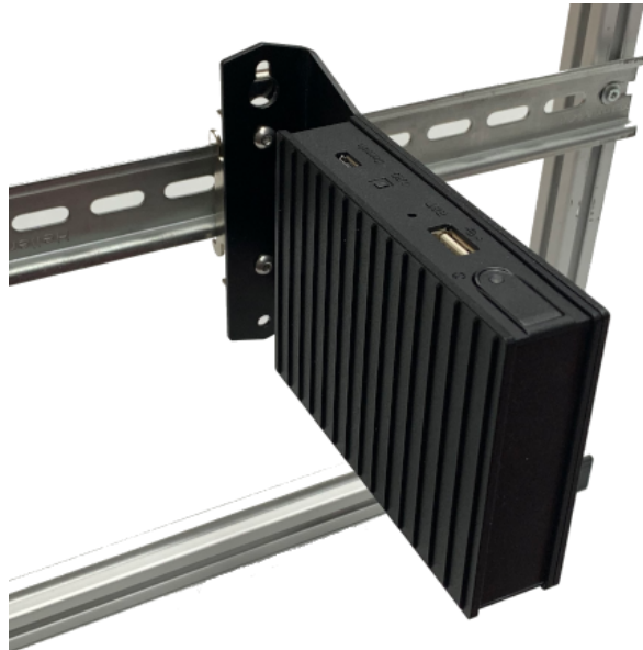
Figure 9: Device mounted on DIN top hat rail
