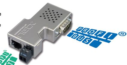
netLINK PROXY integrates a PROFIBUS-DP slave into any superordinate PROFINET network. As connector the device is plugged directly onto the PROFIBUS-DP interface of the DP-Slave and connects to the PROFINET network via the RJ45 socket.
