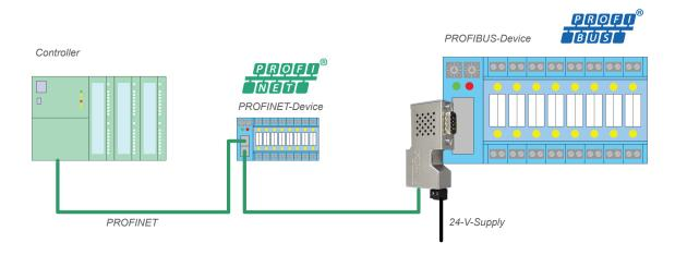
netLINK PROXY is plugged directly onto the PROFIBUS-DP connector of the slave. It is powered by 24 V. The RJ45 PROFINET jack is to be connected to PROFINET. The PROXY is configured via a PC with the configuration tool suite SYCON.net.
