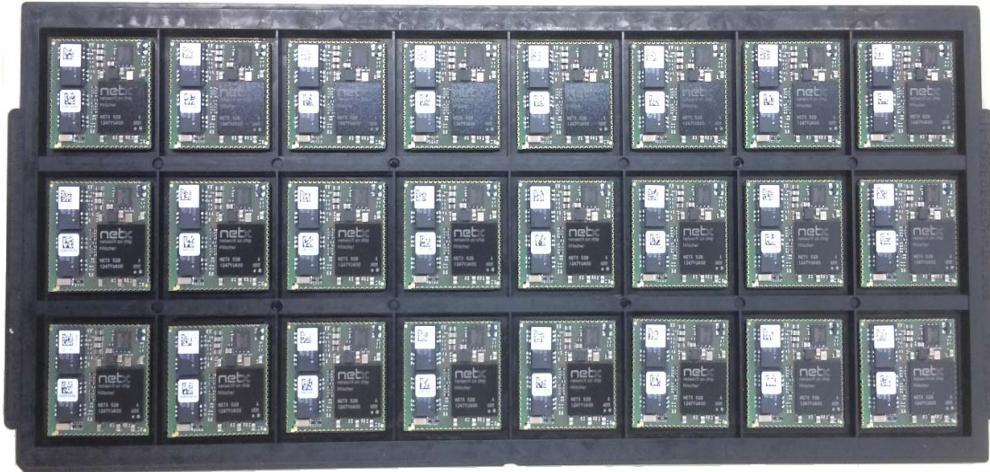
Figure 2: netRAPID tray containing 24 pcs. for series production
